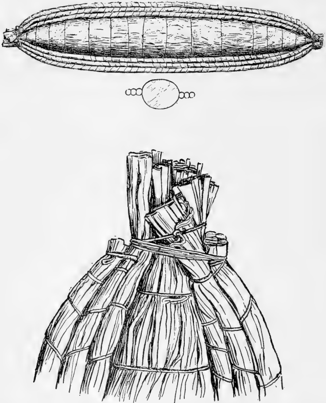
FIGURE 21.—Totora balsa, Guanacache Lagoons. Top : Balsa, full length and cross section. Bottom : Detail of end of balsa. (After Métraux, 1929, p. 4 and fig. 5.)
